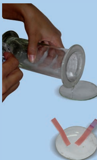
Fig. 4.4 (b) : Testing of solution with litmus papers
